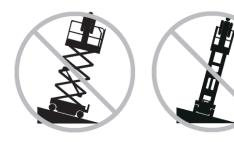
Do not depend on the tilt alarm as a level indicator.
